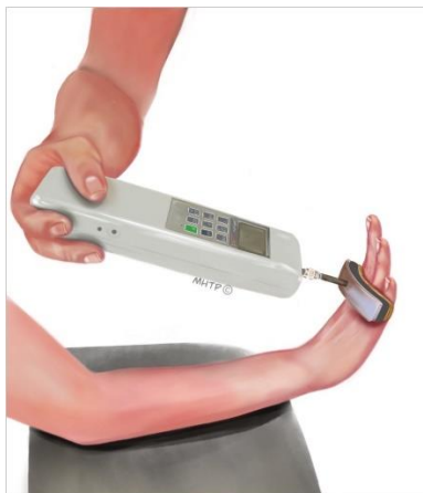
Figure 4. Wrist extension measurement using an electronic push/pull dynamometer (EPPD).
