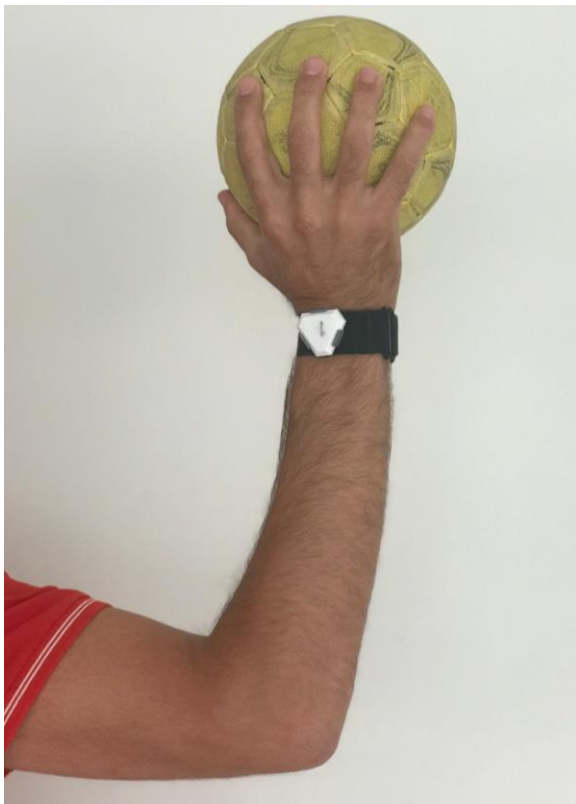
Figure 2. Demonstration of Throwing the Ball with Wrist-Mounted Accelerometer
