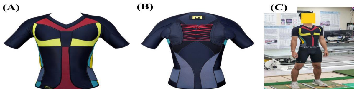
Figure 2. Functional garment design and application. (A) Front view of the functional garment designed for posture maintenance and spinal correction. (B) Back view showing adjustable elastic components for spinal support. (C) Participant wearing the garment during testing.
